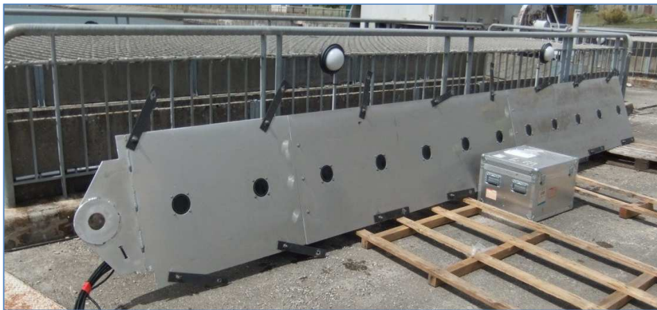
Figure 4. Steel plate carrying 12 ASFM transducers.
