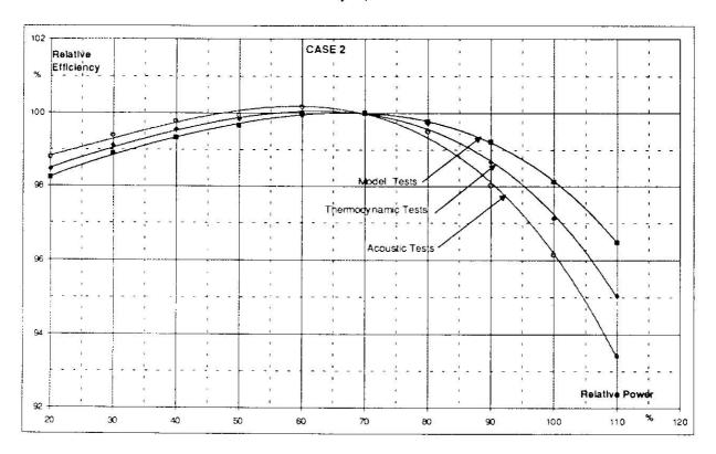
A comparison with model tests, performed on a vertical shaft test rig with an overall systematic error of about  $\pm$  0.20 %, scaled up using the Grein formula, shows a good agreement with the prototype tests till 80%, while at full load the model efficiency is higher than the values determined by means of thermodynamic tests. The efficiency of the model shows a 1.50 % decrease passing from 8/10 to full power.
