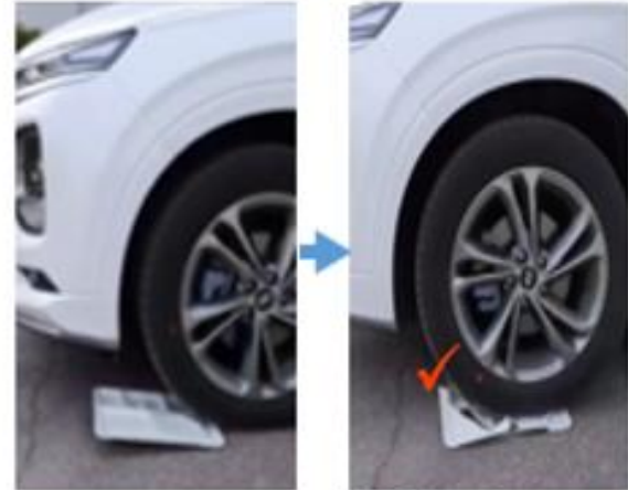
[Current Material food tray Completely Cracked after vehicle load]
