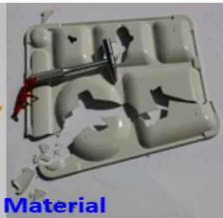
[Current Material food tray Completely Cracked after vehicle load]
