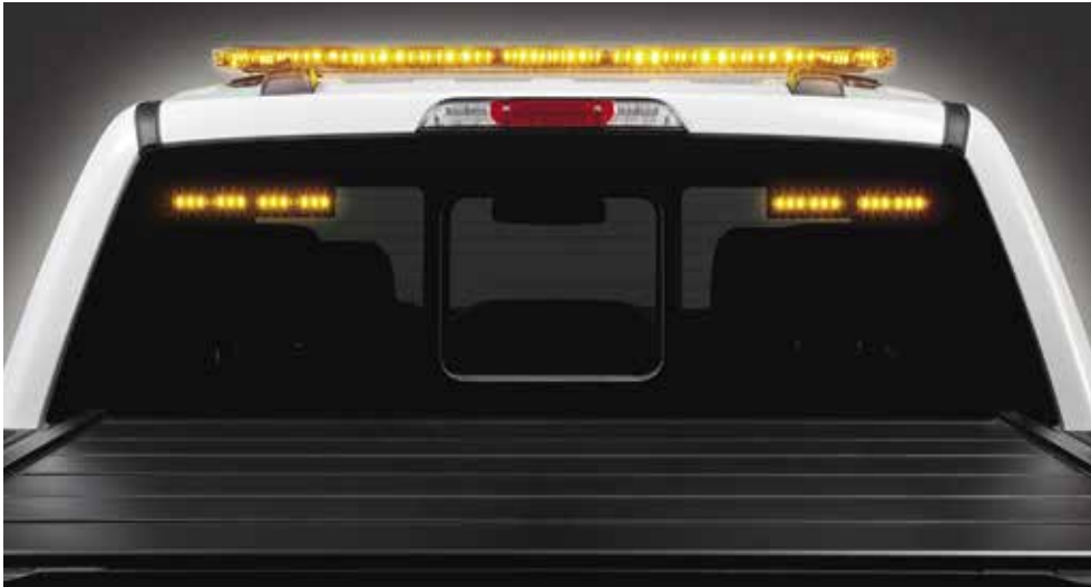
MicroPulse Ultra mounted to rear window using adhesive mount kit
