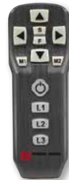
Battery-powered wireless Bluetooth controller
