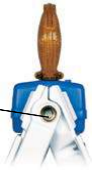
Combination metal hinge/bolt protector (bushing), keeps barricade legs tightly locked together.
