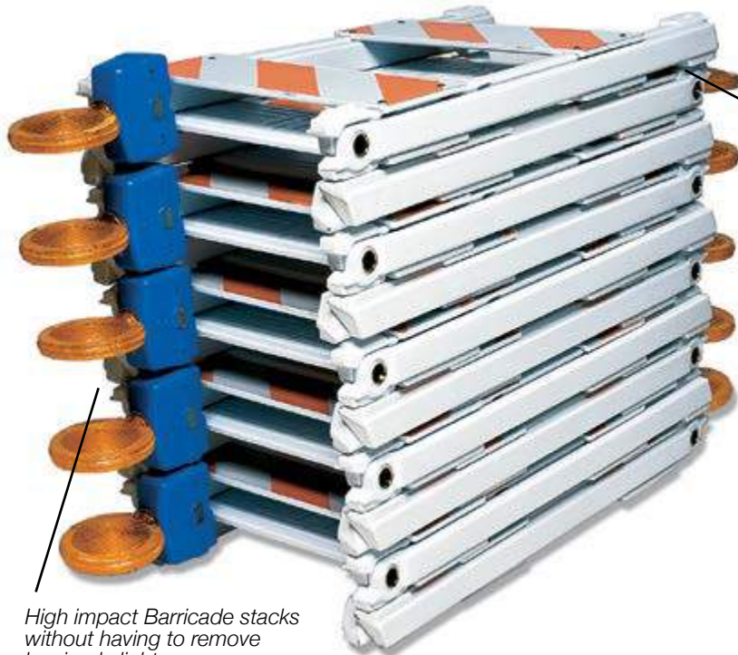
Molded-in male and female stacking lugs keep barricades firmly in place for shipping and storage.
