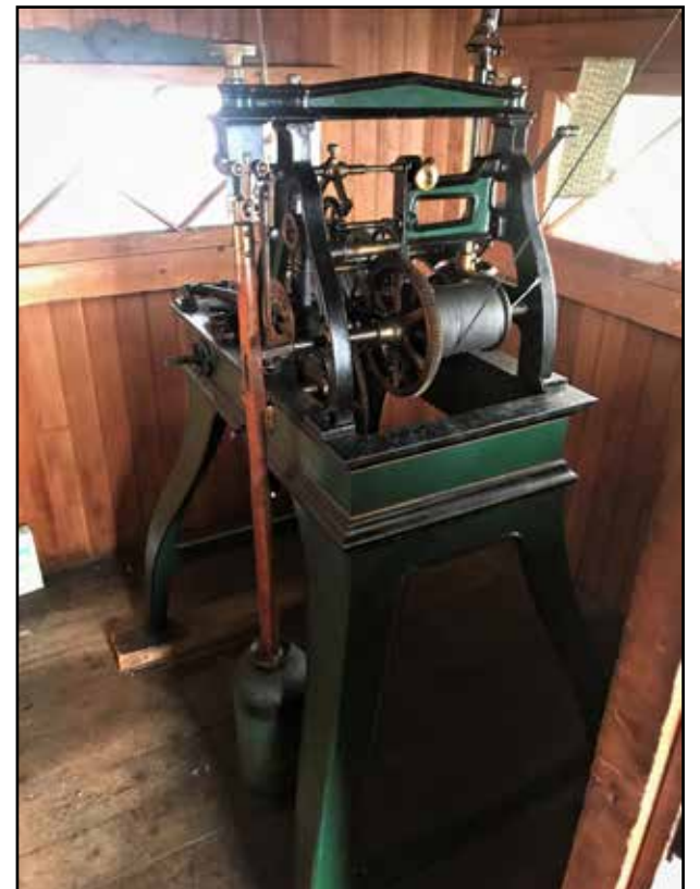
The Redstone Clock's winding mechanism with weights and pendulum.
