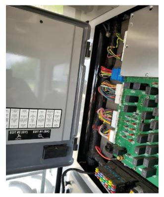
Use the two diagnostic port connections to connect to the Gleaner JD-Bridge. Both of these diagnostic ports are visually the same, so care is needed to make sure the proper connections are made. The main diagnostic port of the Gleaner-JD Bridge (labeled Main) is connected to the rightmost diagnostic port, while the secondary diagnostic port of the Gleaner-JD Bridge (labeled Secondary, and contains only 1 green and 1 yellow wire) is connected to the leftmost diagnostic port.
