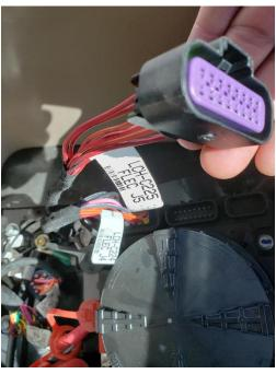
On 2022 and newer models there may be a "VD04" steering controller already installed. This controller can be accessed via a panel behind the drivers seat.
