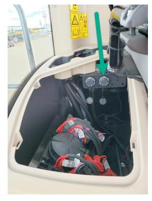
Locate the connector LCH-C225 on the forward side of the round fuse box and disconnect it.
