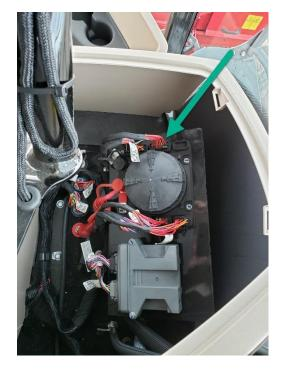
Insert the power adapter cable with the single purple wire here. This connector provides switched 12V power to the Bridge and JD components.
