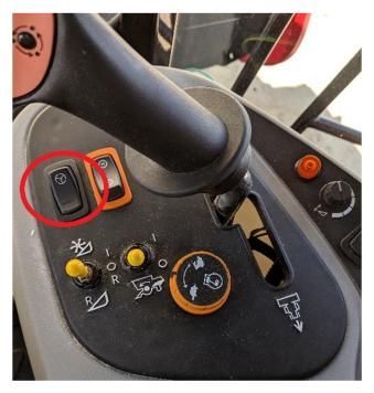
In order for yield and moisture to be displayed on the JD Monitor, a task must be started on the AGCO monitor in the machine.
