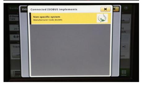
On John Deere 1800, 2600, 2630 the application will be shown in the side menu of the John Deere display. The side menu is opened by clicking the button on the bottom right of the display.
