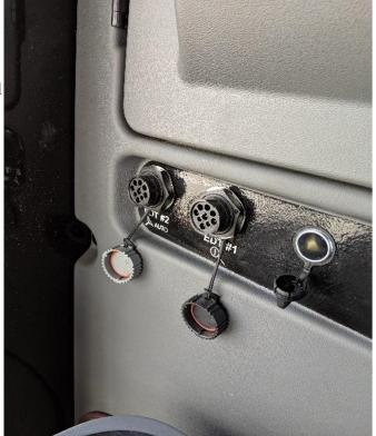
Use the two diagnostic port connections to connect to the MasseyCombine JD-Bridge. The main diagnostic port of the MasseyCombine-JD Bridge (labeled Main) is connected to EDT#2 'AUTO', while the secondary diagnostic port of the MasseyCombine-JD Bridge (labeled Secondary, and contains only 1 green and 1 yellow wire) is connected to EDT#1 diagnostic.
