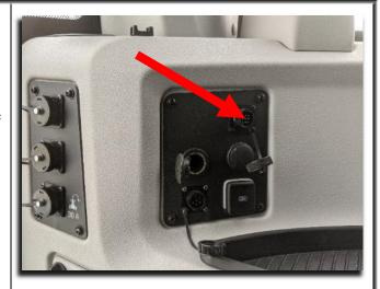
Connect the smaller 9-pin female connector of the Agra-GPS bridge to machine adapter into the 9-pin male ISO connector of the machine.
