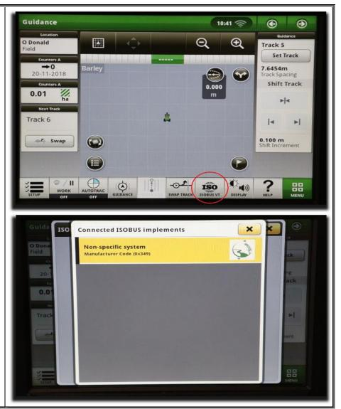
On John Deere 1800, 2600, 2630 the application will be shown in the side menu of the John Deere display. The side menu is opened by clicking the button on the bottom right of the display.
