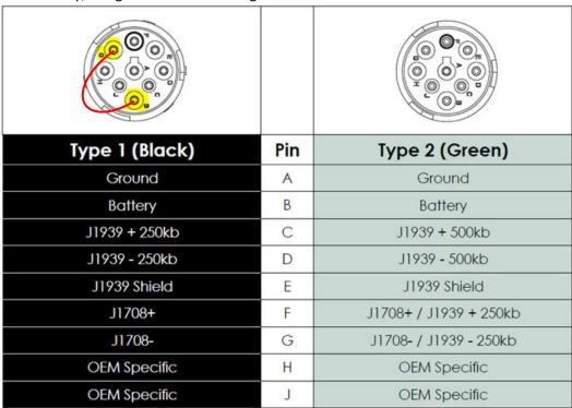
Here an example to bridge Pin B and G without bridge connector:
