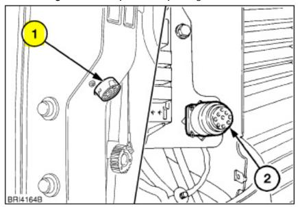
Alternatively, bridge Pin B and G of diagnostic socket 1.
