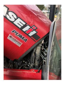
Remove the existing 2-pin connector from the valve block and connect the 2-pin from the adapter. Secure the cable away from any heat source and moving parts. Use plastic cable ties.
