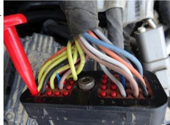
Use the 1<sup>st</sup> adapter which has the black 12-pin deutsch connector, the big black 40-pin deutsch connector and the long cable to the 2-pin deutsch (DT).
