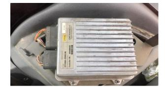
Use the red deutsch removal tool, to remove a connection on the 24-pin deutsch connector and repin them to the 40-pin deutsch on the same cable.
