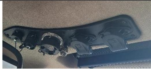
The harness for the JD display connects to the 9pin incab iso connector. They are available at the front and back roof panel connections.
