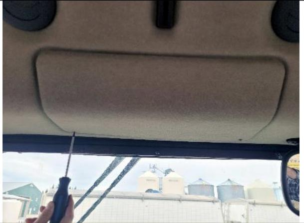
Removing the cover, exposing the 2 layers of metal brackets. The CRG is installed at the upper bracket. VD03 or VD04 steer controller (white box) must be removed. Also a Novatel or Trimble receiver if the tractor was equipped with GPS receiver must be removed.
