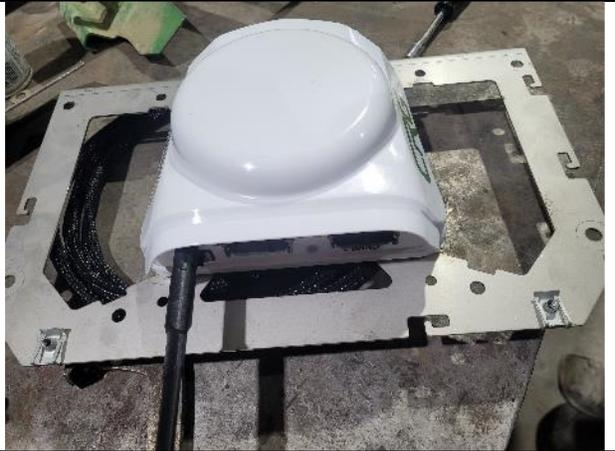
The CRG comes with a build in modem (CRG-JD-WM option) and ships with a cell phone antenna. Some 1167 have a cell phone antenna for RTK correction and this antenna may be used for the CRG. Find the SMA connector from the roof antenna and connect to the CRG.
