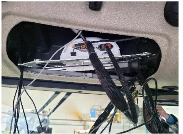
Move the top bracket back into its original position. Note: If you use the Fendt cell antenna, make sure its connected first, otherwise make sure to attach the CRG antenna!
