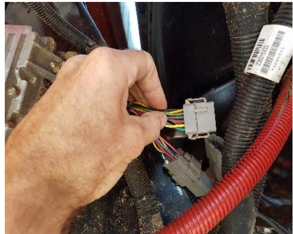
The 2<sup>nd</sup> part of the adapter inserts into the 12-pin deutsch connector going to the seat.
