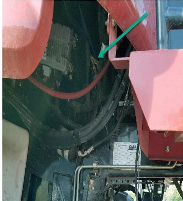
Open the connection the Navcontroller and insert the 12-pin DTM from the Bridge here
