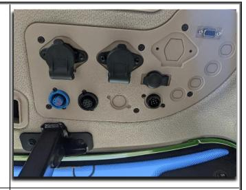
Insert the circular 9-pin female end of the monitor to machine adapter into the 9-pin male ISO in-cab connector.
