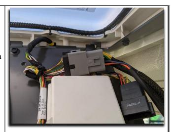
Insert the **Bridge** labelled 12-pin male Deutsch end of the bridge to machine adapter cable (12-pin Deutsch male to 12-pin Deutsch male cable) into the grey 12-pin Deutsch female end of the Agra-GPS AGCO-JD Bridge.
