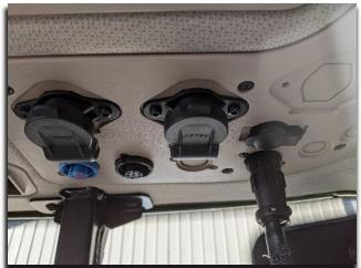
Insert the 3-pin male connector into one of the two 3-pin female power connectors.
