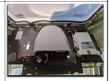
Locate the x4250\_P connector (shown right) and disconnect the female connector from the male connector.
