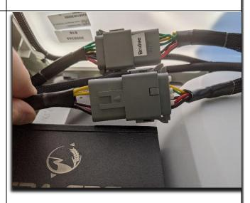
(Connection from the bridge to GPS adapter cable to a StarFire 6000 receiver)
