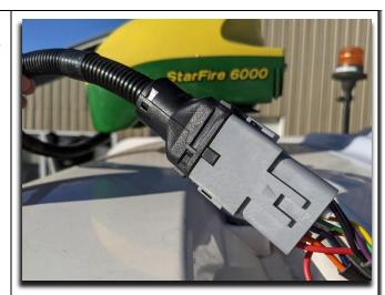
Finally, connect the 3-pin Deutsch male end of the bridge to machine adapter into the 3-pin Deutsch female end of the bridge to GPS adapter.
