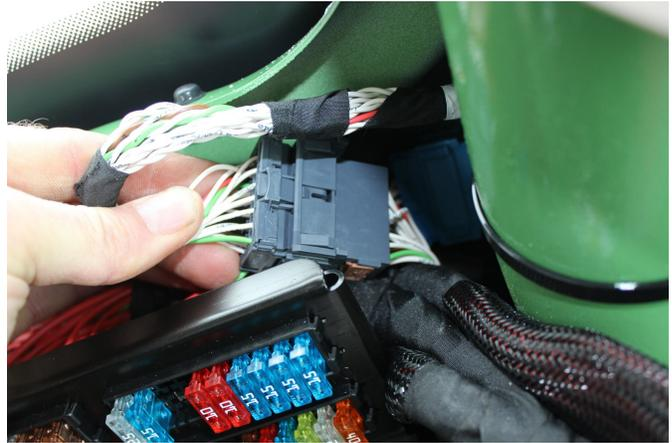
The ground wire (black) should be connected to
