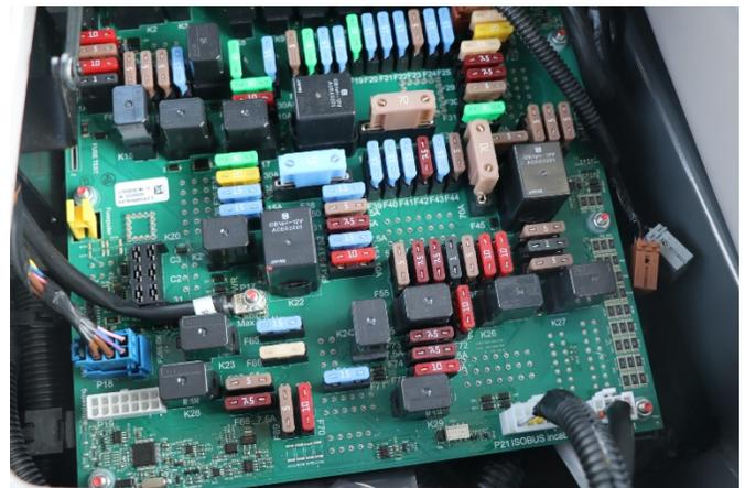
Unplug the ISOBUS connector harness on the circuitboard. The 6-pin JPT female TE 1-965640 (blue plug) connects to the 6-pin JPT male blue plug on the circuitboard. The 6-pin JPT male (brown plug) connects to the 6-pin JPT female of the ISOBUS connector harness that was just unplugged.
