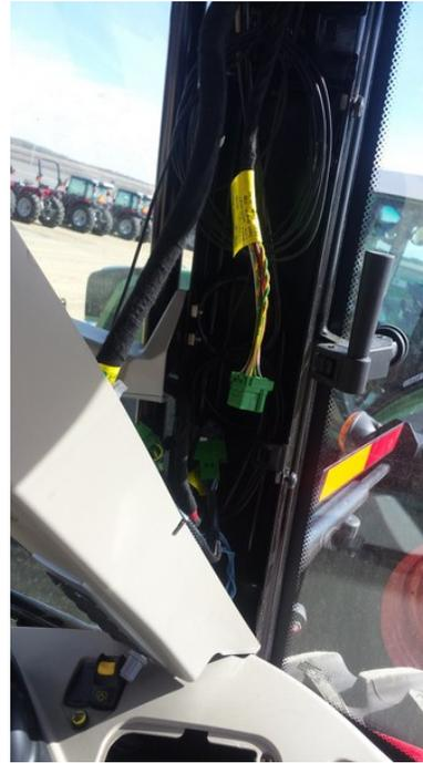
From the adapter cable (right picture), connect the green female connector with the green and yellow cables to the now open connector X282 in the Massey. The cable connector going to the roof remains open!
