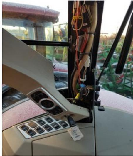
The connector is marked X282. Open the connector and use the adapter provided with the Bridge. The other side of the connector goes to the roof components which are not needed when working with the JD GPS, so this side of the connector remains open.
