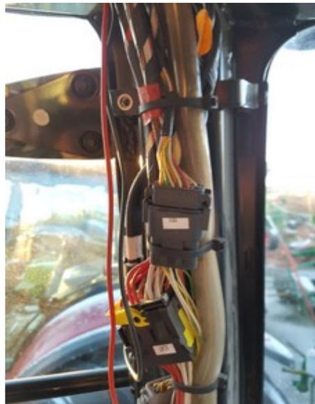
The adapter connects the JD-Bridge with the X282 connector. The red wire must be connected to a 12V constant (battery) power source. A 3 amp fuse is sufficient.
