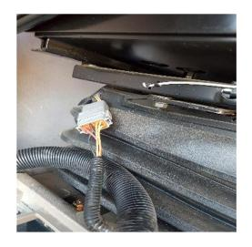
If there is a Trimble NavController installed make sure that is unplugged. The NavController is located outside under the cabin on the right side.
