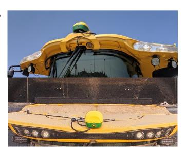
The JD 2630 or 2600 should be mounted that the operator can access the display from his seat. Hide and secure the cable to the JD components.
