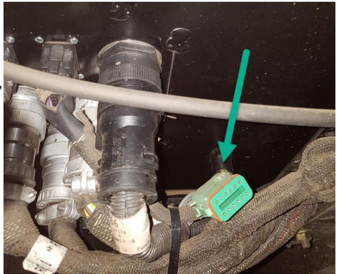
Find the 3-pin deutsch for the wheel angle sensor.
