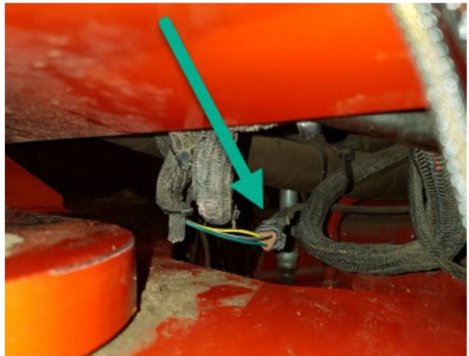
Find the Sauer Danfoss valve with its 4-pin valve connection and the 3-pin transducer connection.
