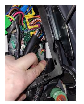
Unplug the ISOBUS connector harness on the circuit board. The 6-pin JPT female TE 1-965640 (blue plug) connects to the 6-pin JPT male blue plug on the circuit board. The 6-pin JPT male (brown plug) connects to the 6-pin JPT female of the ISOBUS connector harness that was just unplugged. It is in the middle of the board.
