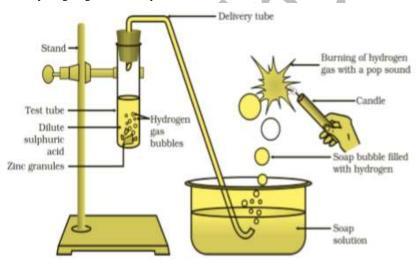
Take few pieces of zinc granules and add 5 ml of dilute H2SO4. Shake it and pass the gas produced into a soap solution. The bubbles of the soap solution are formed. These soap bubbles contain hydrogen gas.
