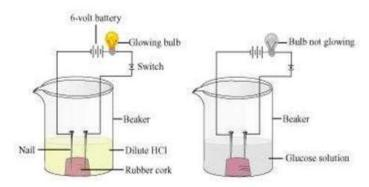
**Result:** HCl dissociates into  $H^+$  and Cl – ions. These ions conduct electricity in the solution resulting in the glowing of the bulb. On the other hand, the glucose solution does not dissociate into ions. Therefore, it does not conduct electricity.
