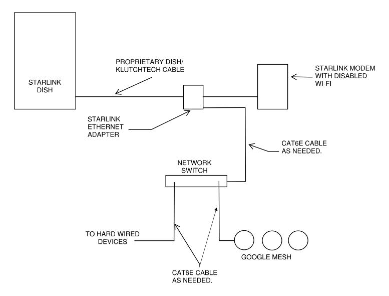
THIS DRAWING REPRESENTS THE BEST, ALL AROUND, INSTALLATION WE HAVE RUN ACROSS. IT UTILIZES THE STARLINK INTERNET CONNECTION AND SOME WIDELY AVAILABLE PARTS THAT IS SIMPLE TO INSTALL AND MAINTAIN FOR THE MOST RELIABLE NETWORK CONNECTION. ALL PARTS ARE AVAILABLE ON OUT WEBSITE. IF YOU NEED HELP, PLEASE FELL FREE TO REACH OUT, SUPPORT@DISHACCESSORIES.COM
