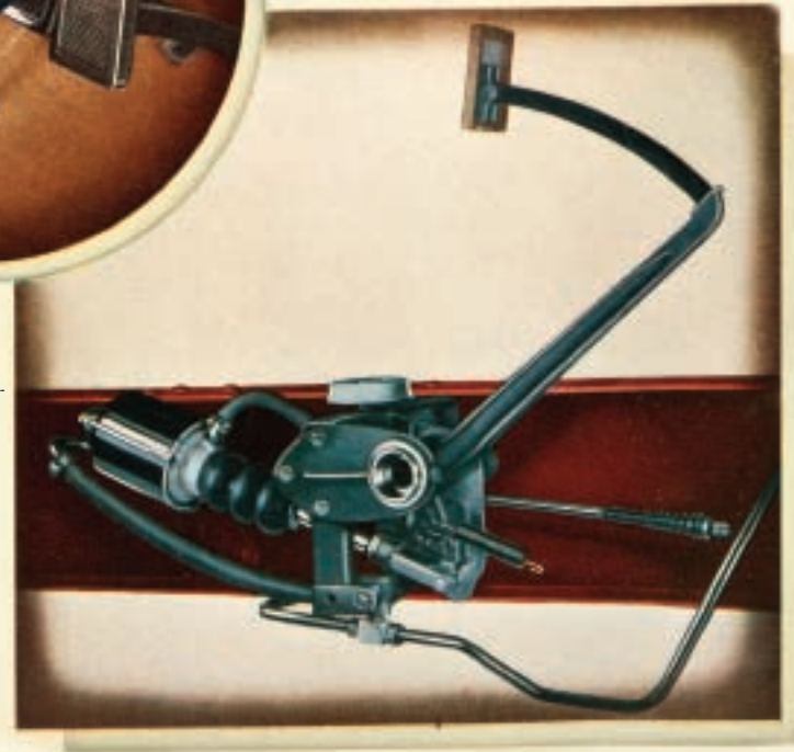
"Booster" assistance on the Packard Twelve gives easy command over its greater power. As shown here, the clutch has a vacuum assistor and a vacuum device also "boosts" break control.
