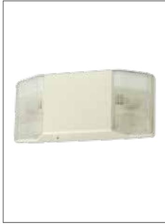
**LOW-PROFILE EMERGENCY LIGHTS** feature flame-resistant, high-impact thermoplastic housings. Universal mounting (with “EZ” quick connects), push-to-test switches, solid-state chargers, low-voltage disconnects, and power-on LED indicator lights are standard. Fixed or fully adjustable, glare-free dual lighting heads are included. **BELR2** has remote capabilities of up to 11 lamp watts. UL listed for damp locations. 120/277 VAC. Five-year warranty.
