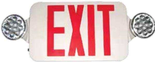
**COMBO MICRO LED EXIT SIGN & EMERGENCY LIGHT** features high-impact thermoplastic construction and a snap-fit faceplate. It comes with field-replaceable chevrons and a universal mounting knockout for J-boxes. Other features include adjustable, glare-free lighting heads; test switch; status indicator; and NiCad battery. UL listed for damp locations. 120/277 VAC. Five-year warranty.
