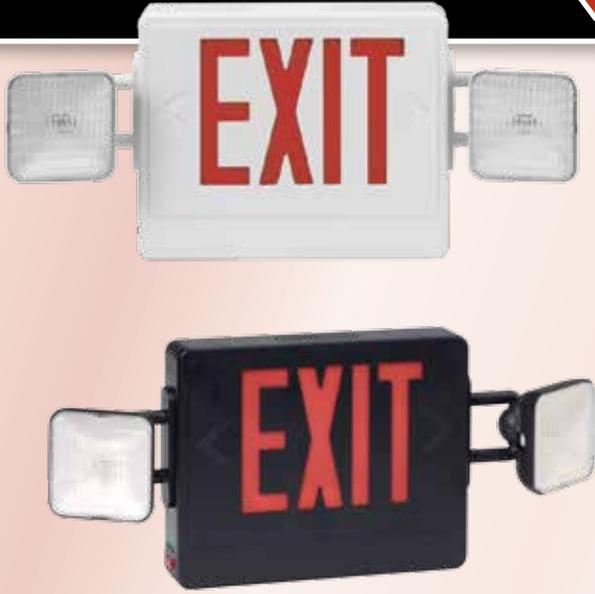
**COMBINATION LED/INCANDESCENT UNITS** meet both exit sign and emergency lighting needs in one economical unit. Their low-profile design comes in a neutral finish, assembled in an injection-molded, flame-resistant, high-impact thermoplastic housing. They also feature a solid-state charger, universal mounting, push-to-test switch, low-voltage disconnect, LED indicator, and universal pop-out chevrons. UL listed for damp locations. 120/277 VAC. Five-year warranty.
