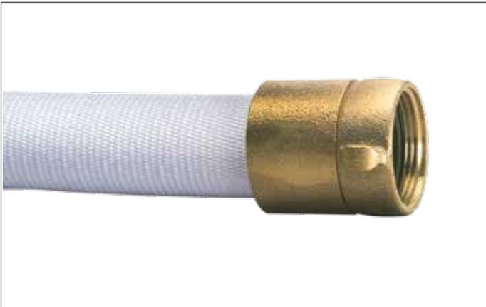
This **SINGLE JACKET FIRE HOSE** has a proof test pressure of 500 psi and a service test of 250 psi. It features 100% polyester rubber-lined material for extra strength and flexibility. FM approved.
