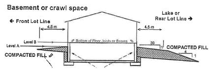
Foundation must be reinforced concrete able to withstand hydraulic pressure and ice action Windows & other well openings must be protected as needed unless builder designs for and accepts interior flooding. Sump pumps and other special plumbing may be required.
