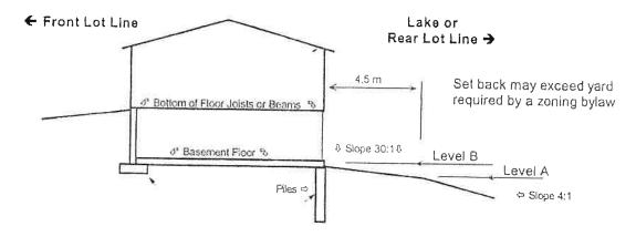
Foundations must be reinforced concrete able to withstand hydraulic pressure and ice action Windows & other wall openings must be protected as needed unless builder designs for and accepts interior flooding. Sump pumps and other special plumbing may be required.
