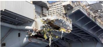
USS Truman collision damage starboard side aft
