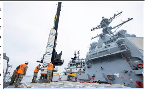
Sailors aboard the USS Spruance (DDG 111) guide training ordnance into the ship's forward vertical launch system (VLS) cells during a proof-of-concept evolution in San Diego. MV Ocean Valor conducted its first at-sea vertical launch system reload with Spruance, demonstrating the ability to re-arm surface vessels who employ VLS. (U.S. Navy photo by MCS 3rd Class Taylor Crenshaw)
