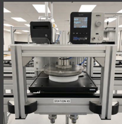
Automated Leak Testing
