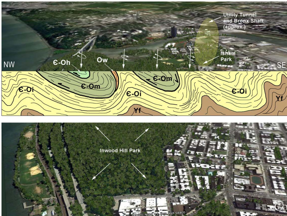
Figure 19 - Oblique northeastward Google Earth terrain view of northern Manhattan and The Bronx with Dyckman Street near the edge of the lower section. Interpretive geological section in cut-away slice roughly across Isham Street in Manhattan. Proposed along-strike correlation between Isham Park and the Bronx Shaft of the a utility tunnel (approximately located for security reasons) shown in yellow shading marks the along strike extension of the SE-dipping limb of an overturned SW-plunging F_3 antiform. Note the positions of major overturned F_3 antiforms and synforms (shown in white), the folding of sheared lithologic contacts, and the position of a thin slice of Walloomsac Schist (Ow) in Inwood Hill Park.
