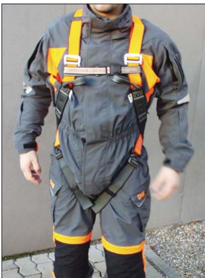
PSE Fall arrest system Personal safety equipment Consisting of mobile runner, harness, self-locking snap-hook, guided type fall arrester, rope bag.
