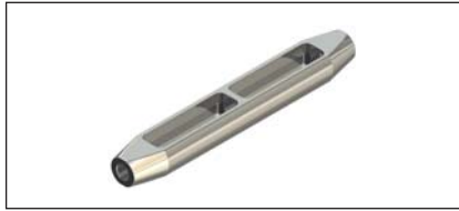
Tensioning element Allows checking of the pretensioning of the steel rope, stainless steel AISI 316L Min. breaking load >40 kN
