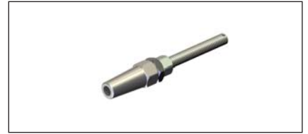
Tensioning terminal with left-hand thread Stainless steel AISI 316L, Min. breaking load >40 kN
