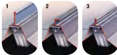
The Pittsburgh double-lock standing seam produces exceptional weathertightness.
