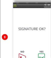
9 Depending on the acquirer configuration the terminal might request to check the customer signature and press the green key.
