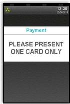
If more than one contactless card is presented to the contactless card read zone together then the card read will fail. This may occur if the card is presented in a wallet with other contactless payment cards, or other contactless cards such as public transport smart cards. An alert tone will sound and the customer will be prompted to re-present the card.
