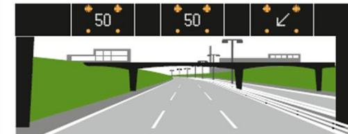
Each lane has its own signal; each signal has two pairs of amber lamps that flash from top to bottom. You should obey the signal for your lane
