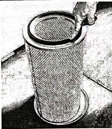
Fig3-14 Rubber Ring Installation
