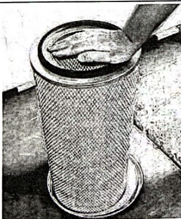
Fig3-14 Rubber Ring Installation
