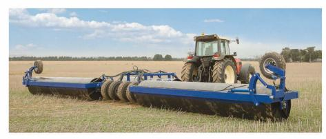
Used for surface crushing and compaction after plowing or after sowing, the working part is the pressure roller. The side roller can folded with hydraulic cylinder. This product adopts hydraulic locking and lifting function, which is convenient for operation. The connecting part of the bearing seat is added with cushioning and locking device, which relieves the impact of equipment during work and increases the service life of the equipment.
