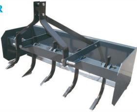
This scraper is perfect for landscaping, levelling, backfilling, and grading. With forward facing rippers to break up the soil and a high carbon steel blad, breaking up and levelling out is achieved in a single pass. A further replaceable rear facing steel blade is available to back fill if required.
