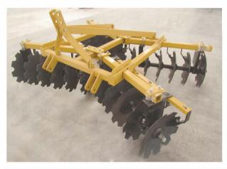
Mainly applicable for breaking up the clods of farmland, light and medium soil after furrow and loosening soil and mixing soil and fertilizer before sowing. With simple structure strong ability to rake; durable, easy to use and maintenance, etc., meeting the requirements of intensive cultivation.
