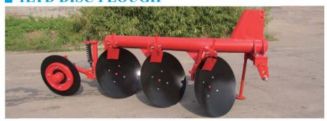
It is designed to work in all types of soil for functions such as soil breaking, soil raising, soil turning and soil mixing. It is used to open the new fields and to process the stony areas. Its special design allows to easier work in rocky and rooted areas. It is specially useful in hard and dry trashy land.
