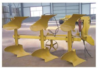
The swivel plow is matched with tractor, and the double-distributor controls the lifting and the turning of the plow. Strong design for all conditions. Big variety of working width choice for all tractors.
