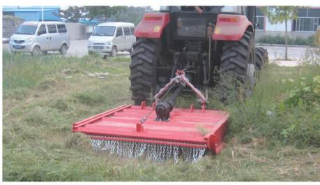
Model 9G mower are suitable for cleaning and slashing in bush and grassland, As well as improving uneven ranch. The machine is scientific in design, durable in service, easy to operate and maintain, adjustable in cutting height and has excellent working performance. They are more ideal agricultural machines for grass slashing and ranch cleaning.
