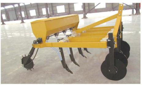
3ZFQ Lawn fertilizer machine is used for grass sowing and fertilizing. It is Suitable for dry granular fertilizer. Front discs open the straw board and the tine point break the lawn less. The tine point cultivating and it put the fertilier into the soil at same time to less the fertilizer volatile loss.
