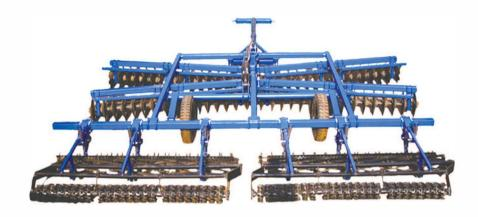
Especially matchable with tractor, Applicable to wasteland, swamp shrub land, heavy soil and stubble land before plouging, breaking clods after plouging, loose soil, can replace the plough on the mature land to carry out the soil plouging operation. The roller is used for breaking up the clods and leveling the ground.
