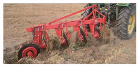
Matchable with tractor, it furrow soil when patches rotate, mainly applicable for complex land, such as weedy land, heavy soil, farmland with bricks and stones, etc. no tied with grass, not obstruction, can cut off stem of crop and overcome bricks and stones, with high efficiency, good quality work, easy to adjust, simple to use, durable,
