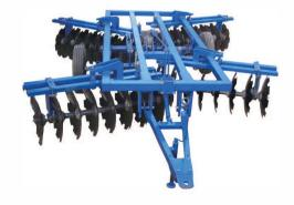
Applicable for breaking up the clods and loosening of wasteland, shrub swamp, heavy soil, can rake the land instead of plough and can also replace the plough on the mature land to carry out the soil ploughing operation. The work efficiency is high, the power utilization is reasonable, and the ability to break up the soil is strong. After the working, the surface is smooth and the soil is loose. It has strong adaptability to the filed with heavy soil, wasteland and weeds.
