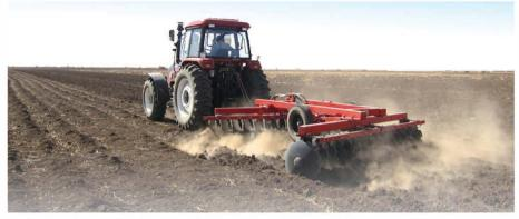
1BZ dragging off-set heavy duty disc harrow is designed for field work as crop residue processing before tillage, Breaking hardened and impervious solid surface, crushing and spreading straw, shattering soil after tillage, planning the land and preserving soil moisture, it can be used on cultivated land for tillage harrow instead of ploughing.
