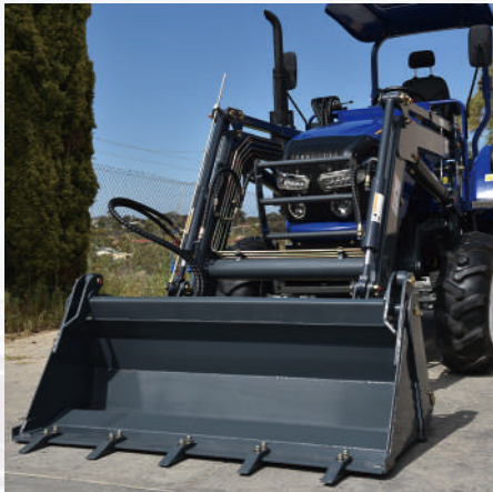
Quick hitch self-levelling front end Loader with 4in1 Bucket (Optional Joystick)
