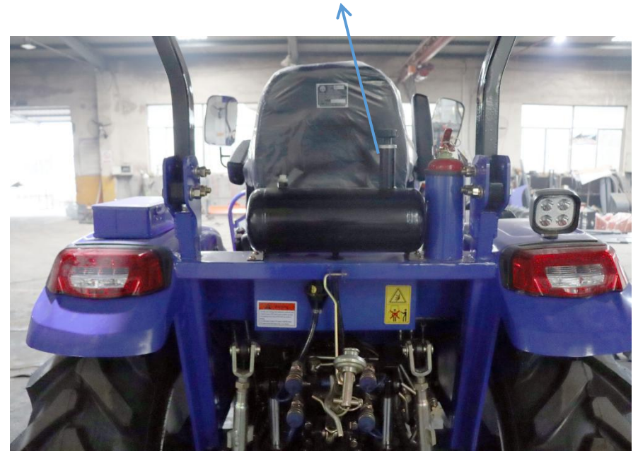
Check&Fill Hydraulic ISO46 Oil Here
