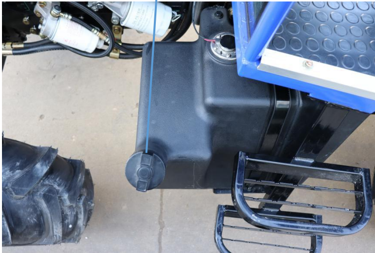
Fuel Tank (Fill Diesel)
