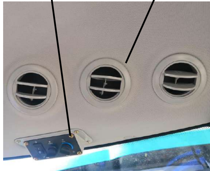
Air conditioner Switches Air conditioner Vents
