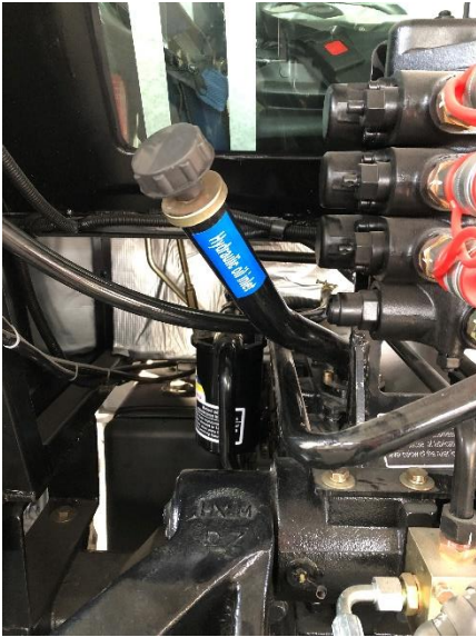
Fill Hydraulic ISO46 Oil Here
