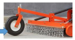
5. Install side place on both side of the slasher and adjust the height as following:
