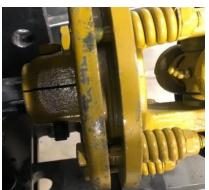
c) Install the PTO shaft on the Slasher gearbox. Refer below;
