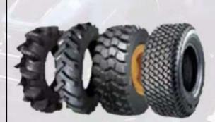
We use TRELLEBO radial tires with front/ rear size of 280/70R20,380/85R24 on Trident 60hp tractor to increase performance, grip & stability. You can also choose from paddy field, grassland and engineering tires according to the working conditions.
