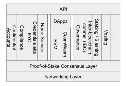
The diagram above shows a high level architecture for Identabitt and the CRDZ Chain. Adapters/libraries are provided in both Typescript and Go for the UX to interface with the CRDZ chain.
