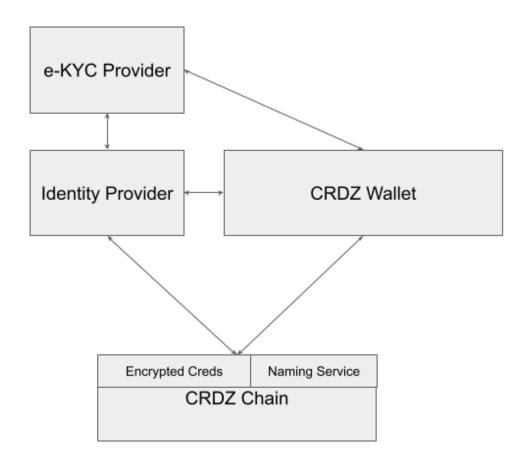
The diagram above shows the external components that a wallet interfaces with in order to perform user authentication (aka KYC). A CRDZ wallet selects an Identity Provider (or more than one if needed for increased decentralization) that will authenticate and certify user credentials. These Identity Providers participate in the CRDZ ecosystem (i.e. they get
