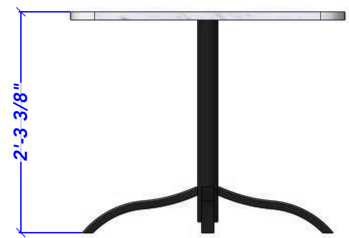
"W" 15 BOOTH TABLE - SIDE ELEVATION
