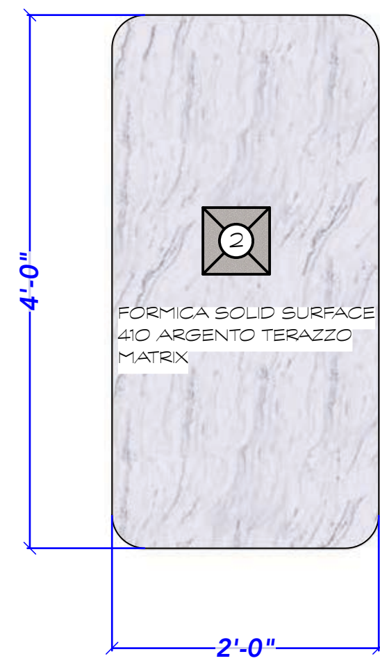
14 BOOTH TABLE - SIDE ELEVATION
