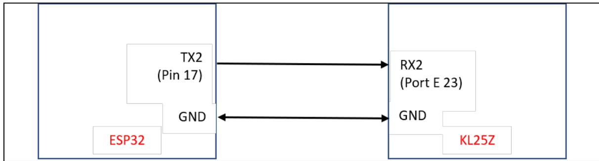
In the Lecture slides, we already went through the process to setup and configure the UART module in the KL25Z. The code implemented the polling approach and this is sufficient for the testing.
