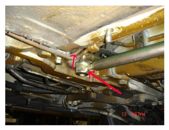
6) Install shift rod original shift rod (or optional 964 424 020 35 shown) onto the transaxle. Make sure to use the shoulder bolt.
