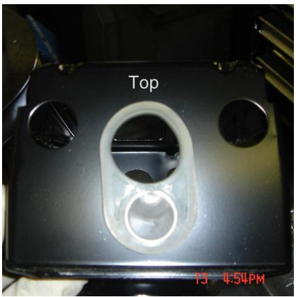
Notice the orientation of the plastic piece. The opening for the shift tube should be towards the TOP of the box.
