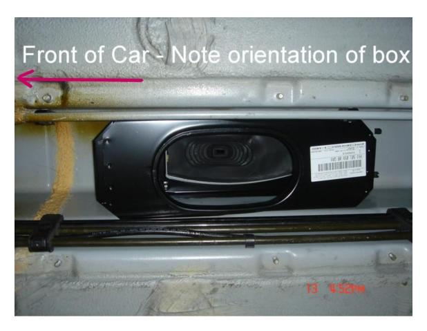
Please not the orientation of the box. There is an offset to the opening in it. This MUST be installed in this orientation. Once in place, weld the box to the tunnel. This will
