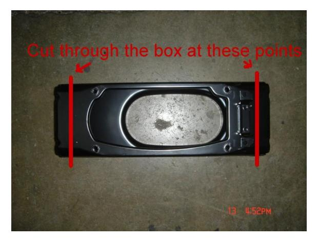
You will need to cut through just the top part of the box. The part between the red lines on the top will be discarded. Now locate where this will go inside the tunnel. This will be where the shifter comes through the car.
