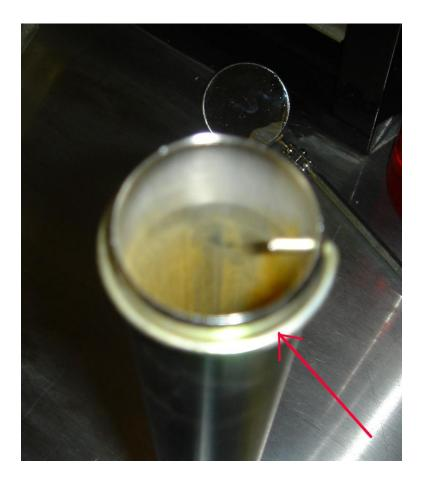
5) Install the front tube (964 424 011 31) to the front ball installed in step one. A c-clamp can be used to make this easier. Be sure to use some grease before assembly.
