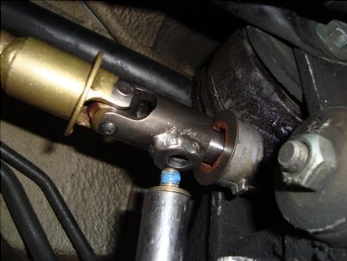
Slide the shift shaft dust boot into place.
