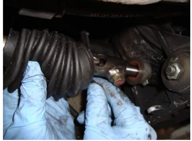
Slide the rod off of the shift shaft. The tolerances are pretty tight and the shift shaft may move. This is okay. No damage can be done and it can end up in any position. The shift lever follows whatever position the shaft is in.
