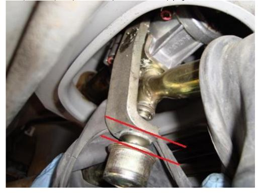
Slide the shift lever (ball end) forward to expose the bottom of the shift fork. This is hard to explain, but move stuff around and it will make sense.
