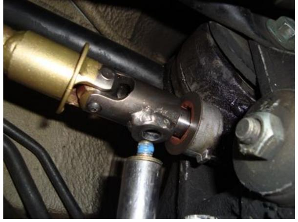
Slide the shift shaft dust boot into place. One end goes over the shift shaft seal on the transmission, the other on the Golden Rod<sup>tm</sup>.
