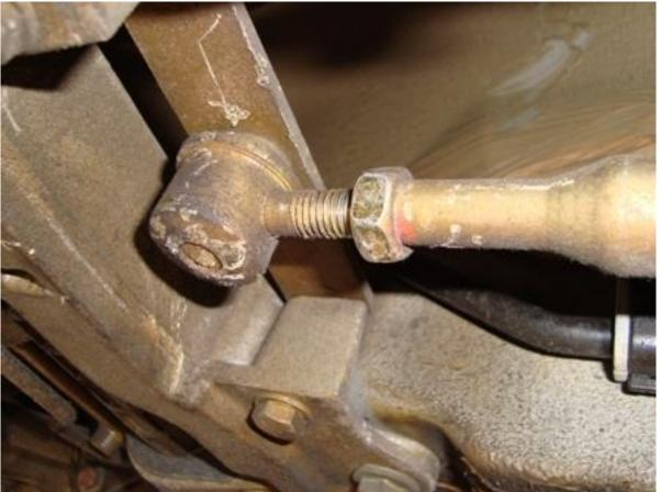
You'll need to remove the front under cover to do this step. Pop the FRONT ball/cup joint apart. Loosen the jam nut. Lengthen or shorten the rod. Lengthening the rod moves the shift lever forward; shorten it to move the lever (in car) rearward. Adjust and then tighten the jam nut.
